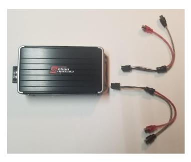
On the amplifier RCA Input Plugs, you will need to separate the RED and the Black plugs like in the picture below.
