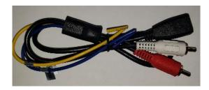
Plug the Extension cable into the back of the Bluetooth, and run the other end down to where the amplifier is going to be installed, then plug it into the Bluetooth Adapter Plug. The RCA plugs on the Bluetooth Adapter Plug will then plug into the amplifier.
