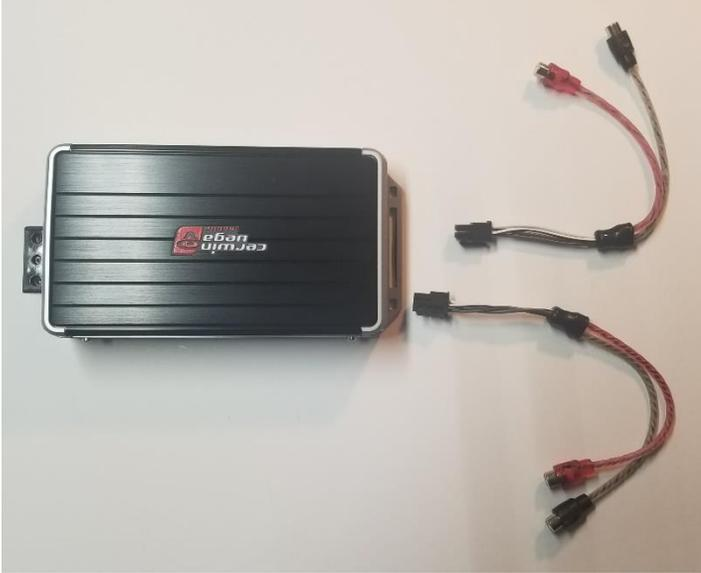
On the amplifier RCA Input Plugs, you will need to separate the RED and the Black plugs like in the picture below.
